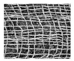
Large-meshed net of 100% hessian, for the application as erosion protection on areas where humus has just been applied; e.g. on pitched roofs, banks, or slope areas.
