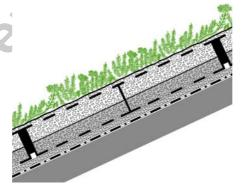
Plant layer "Pitched Roof" System Substrate "Heather with Lavender-light" ZinCo Georaster® Protection Mat WSM 150 Roof construction with root resistant waterproofing
