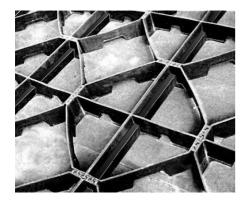
Grid element of recycled polyethylene; applicable shear force protection on pitched green roofs; used as reinforcement for pavings, etc.
